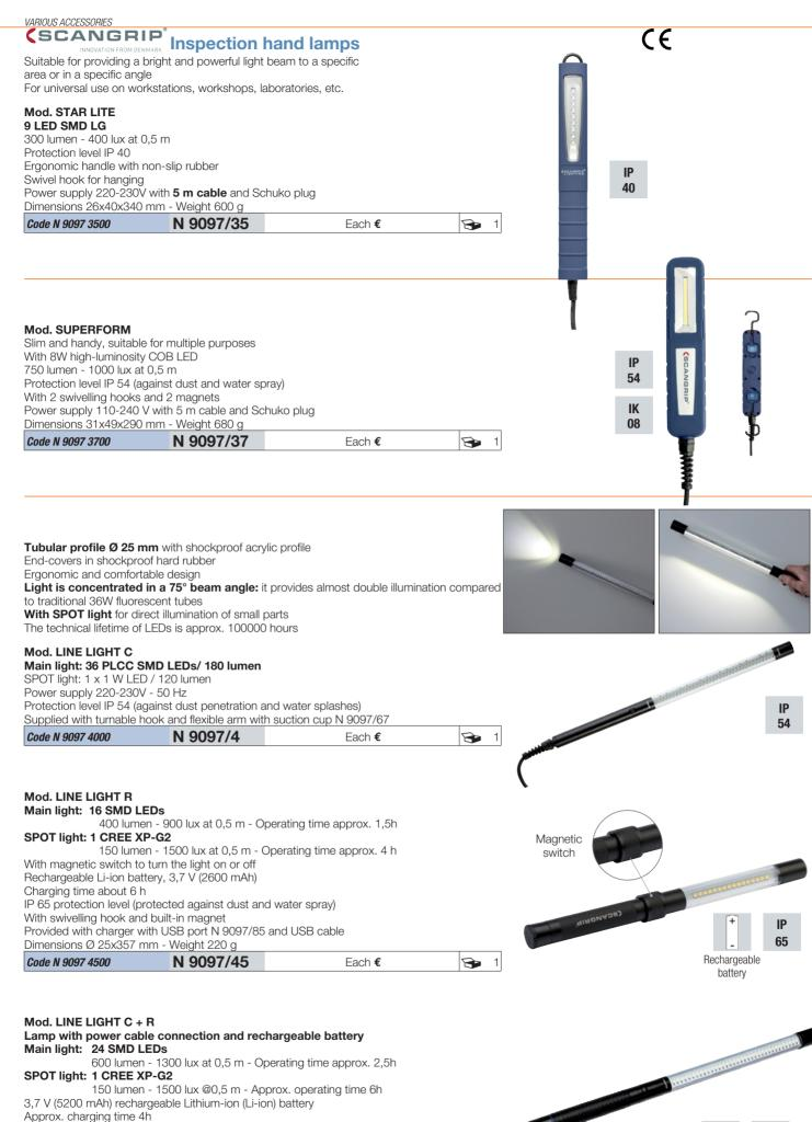
Protection level IP 54 (against dust penetration and water splashes)
