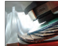
Flexible lamellar flaps for reach corners and edges
